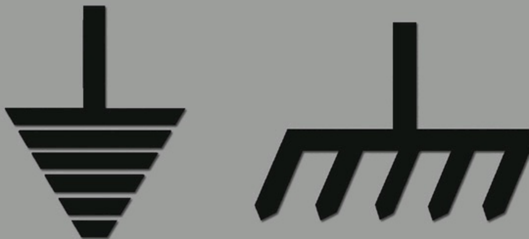
FIGURE 7-6 Two common symbols for grounding that can be found on many pieces of equipment.
